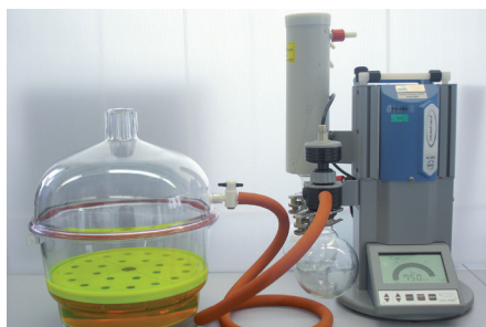
Setup for dye ingress test
