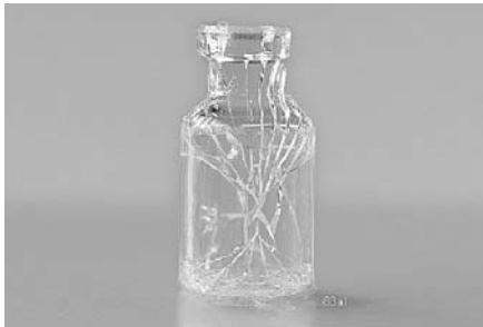
Broken vial after burst pressure test
