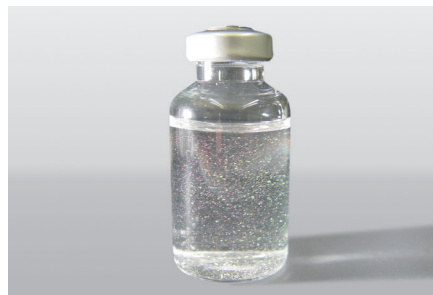
Corrosion effects: glass flakes
