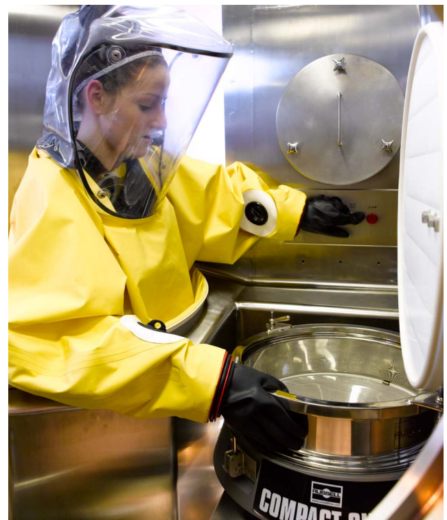
Figure 1. Installation of the Russell Compact Sieve® within the high containment isolator
