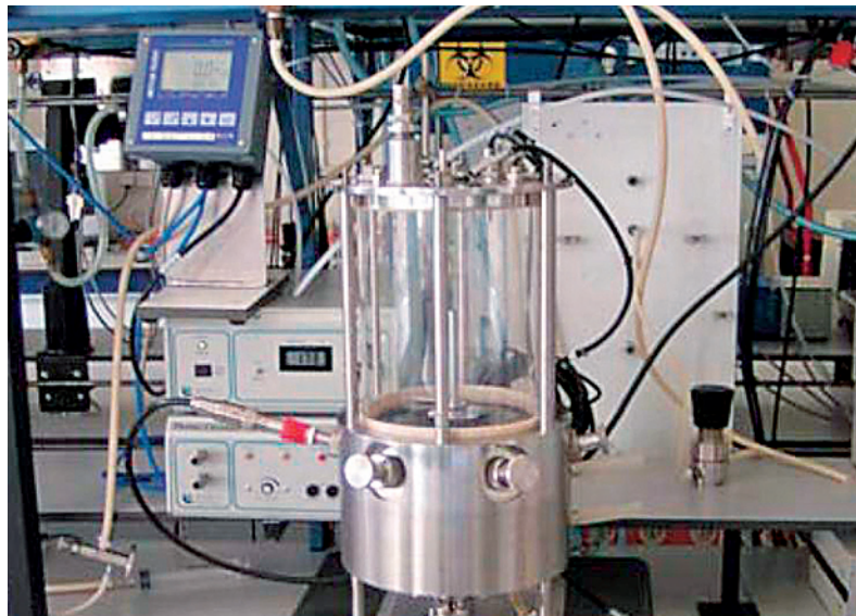
Fig. 1: 4.0 liter laboratory fermenter with side-mounted CO 2 sensor.
